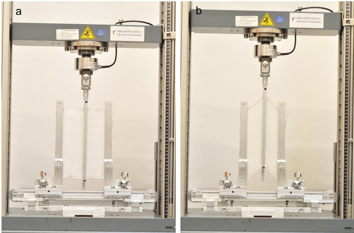
**Figure 4.** The specimen at shear test. a: constant transversal stress and no shearing, b: highly deformed state (transversal stress is still applied)
