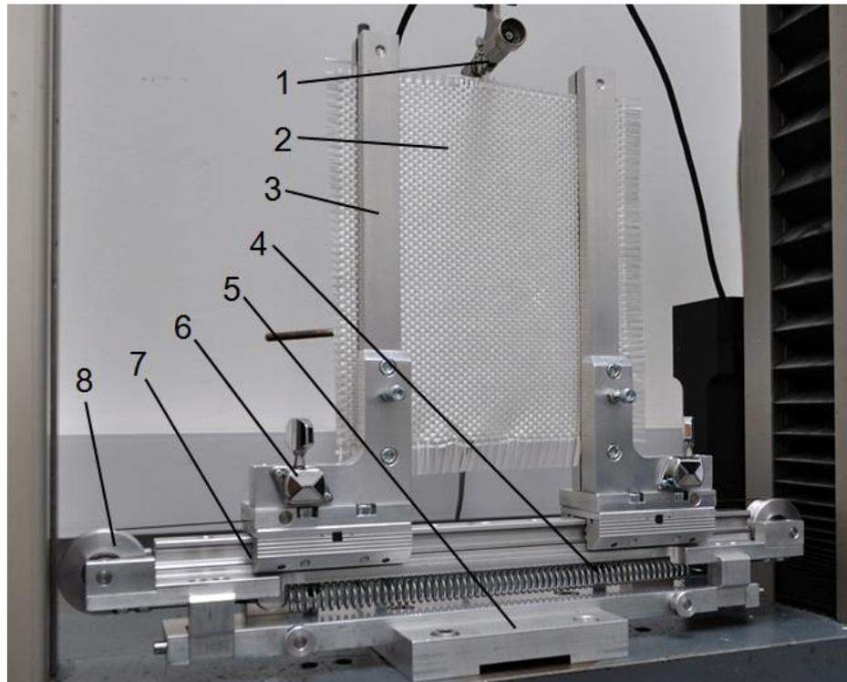
**Figure 3.** The shear apparatus. 1: changeable clamping unit connected to the crosshead, 2: test specimen, 3: clamps, 4: pretension spring, 5: motherboard, 6: gears for adjusting pretension, 7: linear bearing, 8: rollers with bearings
