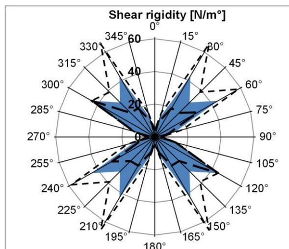
**Figure 6.** Shear rigidity ( $G$ ) of the glass fibre samples as polar diagram (the dashed lines indicate the deviation)
