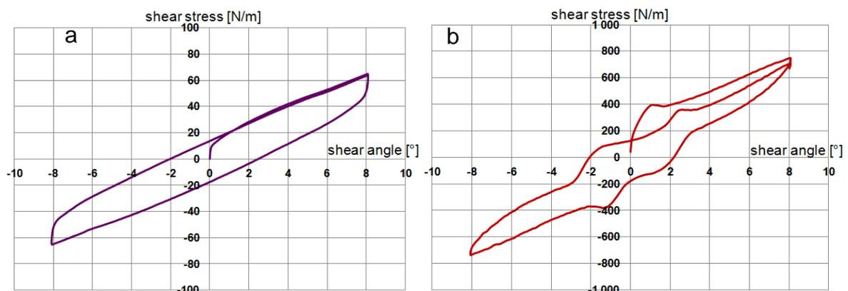
**Figure 5.** Hyteresis test of specimens in  $0^\circ$ (a) and  $45^\circ$ (b) cutting directions
