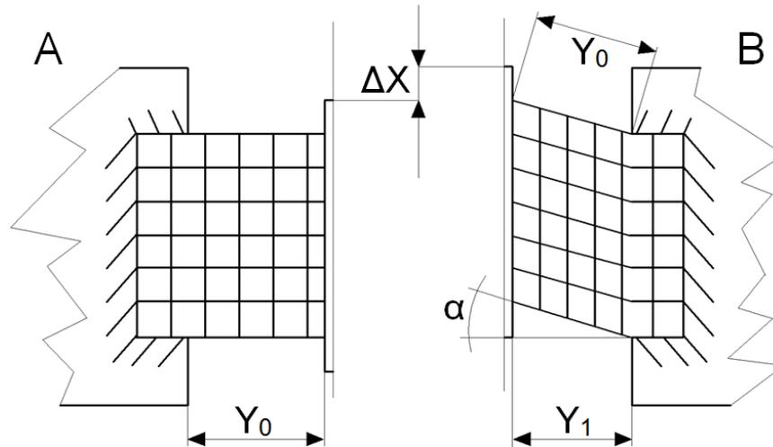
**Figure 2.** The specimen at shear test. A: gripped specimen, B: deformed state during test
