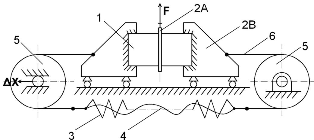
**Figure 1.** The schematic draft of the apparatus. 1: textile specimen, 2A & 2B: grippers, 3: steel spring, 4: HPPE yarn, 5: rollers with bearing, 6: thin rope
